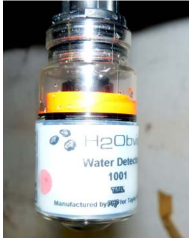
H2Obvious detecting and activating the presence of fluid on the pipe surface under the insulation
