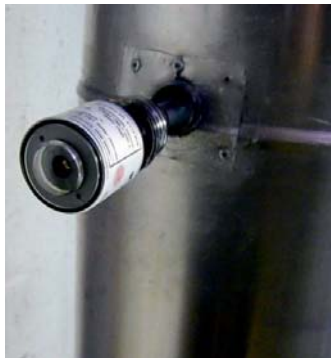
Additional plate to secure the funnel, H2Obvious unit/phial screwed into place (Not essential)
